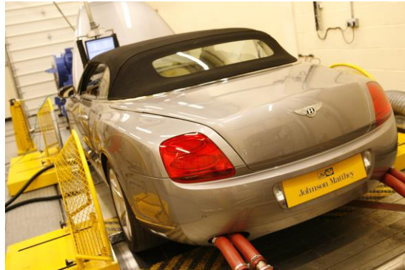
On-road tests re-played in the CVS laboratory multiple times
