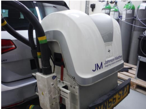
PEMS on-road testing to gather vehicle emissions & ECU data
